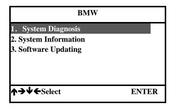
The main menu displays the function menu which is collocated in the mainframe of MOTO-1 BMW diagnostic Scanner. There are three correlative function menus. As shown in the picture above, the black item means the choosing item.
