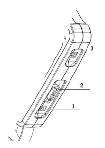
1.power supply insert2.diagnose interface3.USB interface
