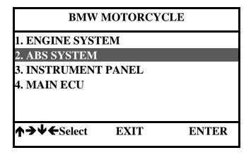
Because there are so many vehicle models and systems, here we make ABS system as an example to explain how to operate. After pressing [ENTER] key, it displays the following interface.
